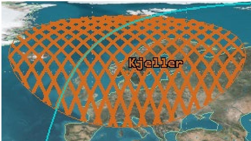
Figure 2: Satellite passes inside the circle for orbital height of 500 km.
