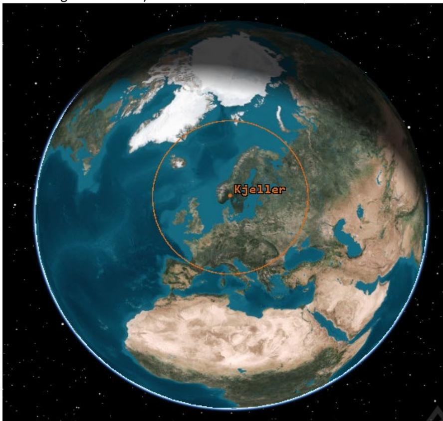
Figure 1: Kjeller ground station and coverage for orbital height of 500 km.
