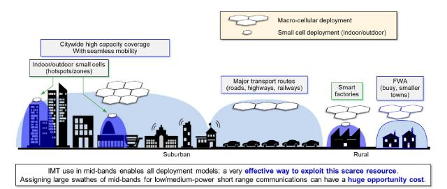
Fig. 1. IMT in bid-bands can address both wider area and local area deployment scenarios cost effectively. Ref: Vendors presentation at the  $2^{nd}$  European 6GHz webinar – Dec. 2021.
