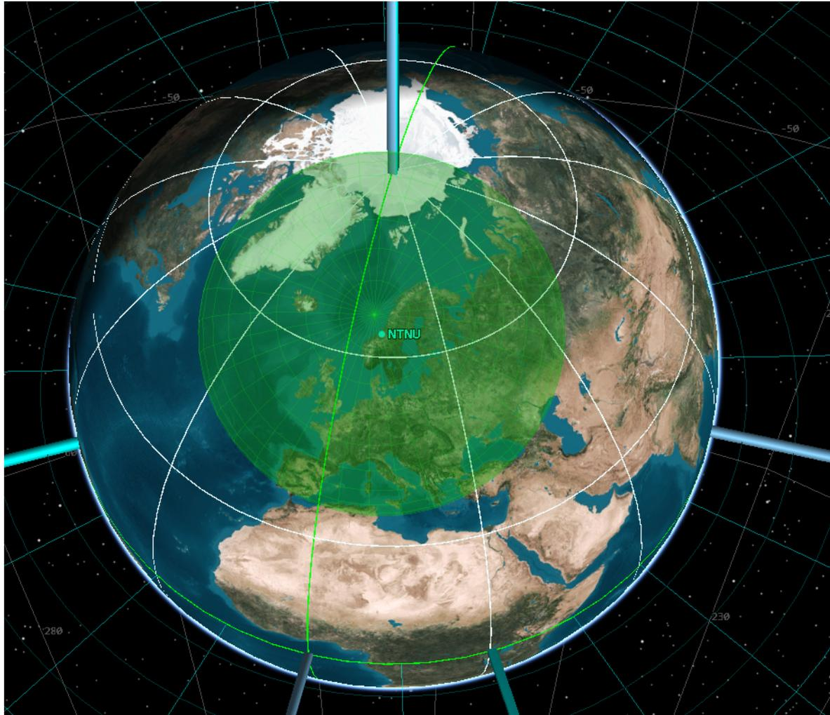
Figure 2: NTNU Ground Station antenna with range 3000 km at 2 deg elevation
