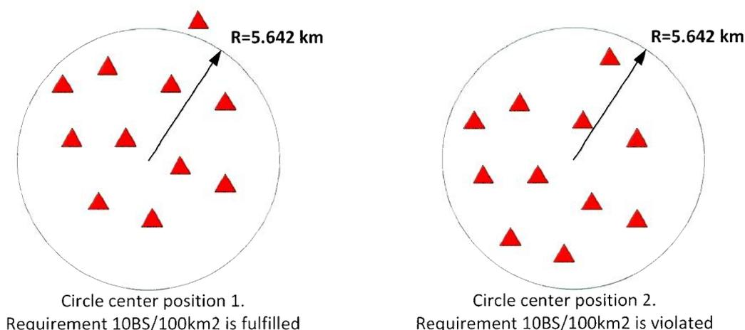
*Fig.A.1. Maximum permissible deployment density calculation*
