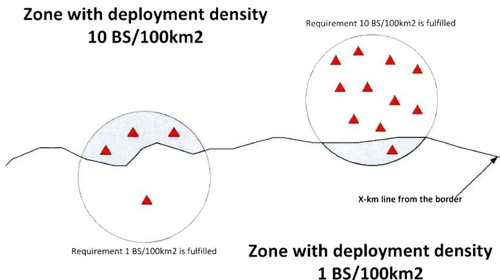
*Fig.A.2. Deployment density calculation at the edge of deployment density zone*
