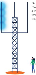
Omnidirectional antennas mounted 1.5 meters out from a triangular lattice mast. One, two or three of the antennas may transmit, and all receive \*
