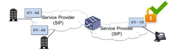
Figure 1: Mechanism for calls between users on SIP-based networks (Source: ATIS)
