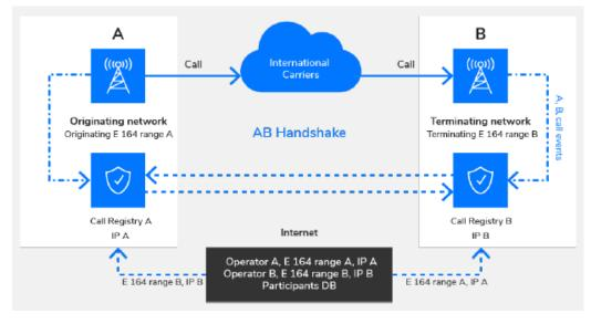
Figure 10: AB Handshake Out-of-Band System Architecture (Source: AB Handshake)
