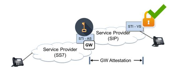
Figure 2: Calls originating from SS7 networks and terminating on SIP-based networks (Source: ATIS)
